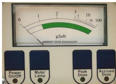
The RM100 and the RM2000 Survey Meter are compact hand held radiation monitors designed to measure x-ray and gamma radiation above 20 keV. The instrument provides an indication of ambient D.E. rate in uSv/hr. The meter may be supplied in two meter scale configurations depending on the model purchased.
